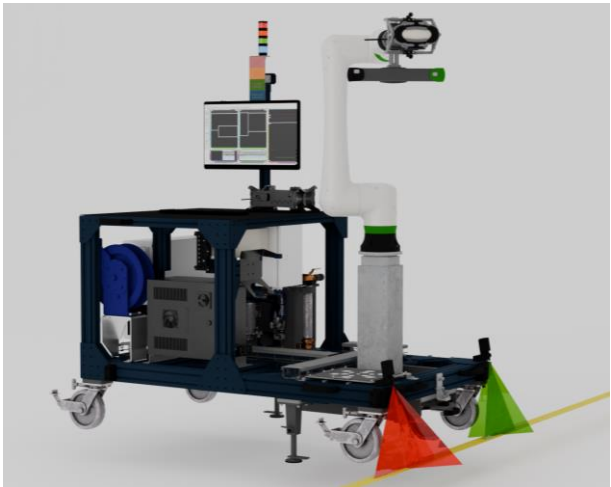
Mobile robotic NDT — repositioned manually by the operator
